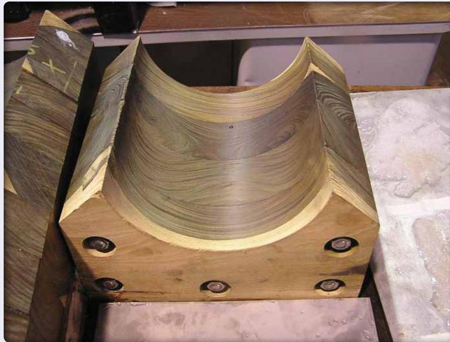
The main turbine shaft bearing at the 4.5-MW Mechanicville plant in New York is made of lignum vitae. The plant has run reliably, 24/7, using this material since it was installed on all six units in the early 1990s. (photo courtesy Albany Engineering Corporation)
